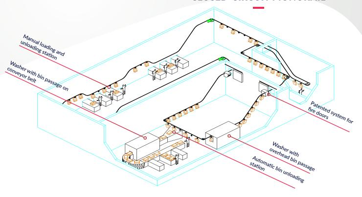
**Calypso is a closed loop monorail conveyor**. It is a simple, clean (designed to be easily cleaned), low-maintenance and silent overhead handling system.
